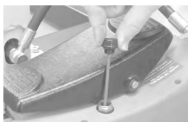
Remove the lid with the gauge to check the oil level
